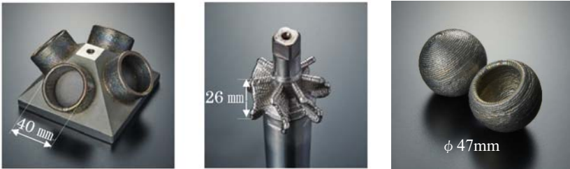
Fig. 4 Examples of dot forming technology
