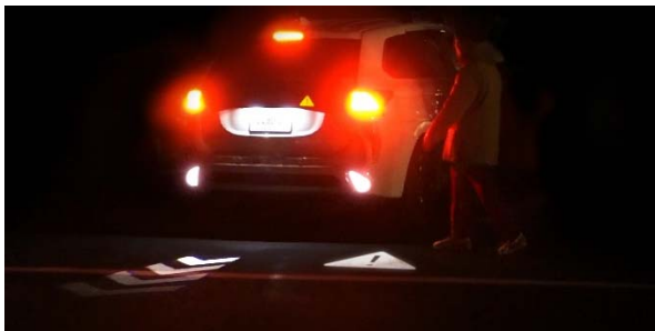
Animated illuminations projected on road surfaces are highly visible even in bad weather
