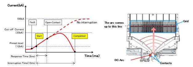
Waveform of a short circuit current interruption
